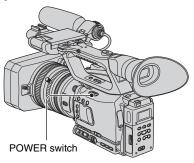
1 Slide the POWER switch to CAMERA or VCR while you press the green button.
