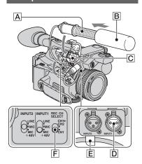
Attach the wind screen B to the supplied microphone A.
